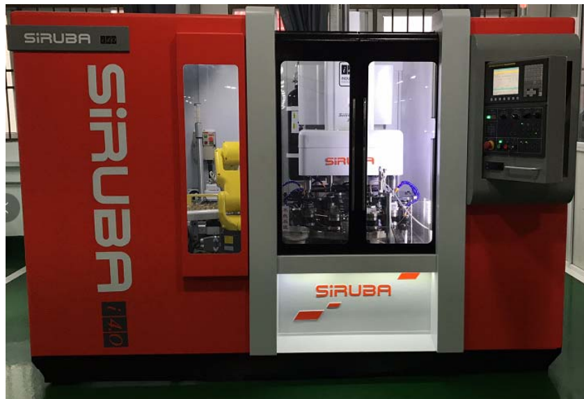
Full auto Honing Machine (independently developed)
