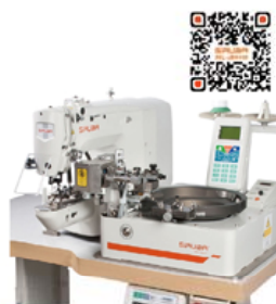
ASP-ABF100J 電子釘扣機附自動送扣 Computer-controlled Lockstitch Button Sewing Machine with Auto Button Feeder
