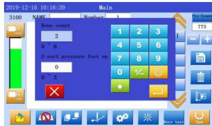
In the main control interface click the parameters box 1, enter the number of bone bits set page. The right keyboard input the actual number of bone bits, press OK to save exit, press Cancel do not save exit
