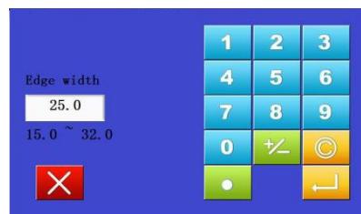
Set the value of the hem height at the main interface by the volume edge width button. (cannot exceed parameter range)
