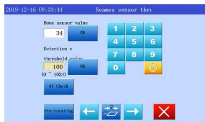
After placing the cloth, click the Send cloth wheel rotation around 3 laps automatically calculate the bone position datum and valve value, click on the key to determine the following value changes
