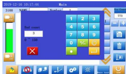
In the main control interface Click the end of the box 3, enter the end stitches count Settings page. The right keyboard to enter the actual number of stitches needed, press OK
