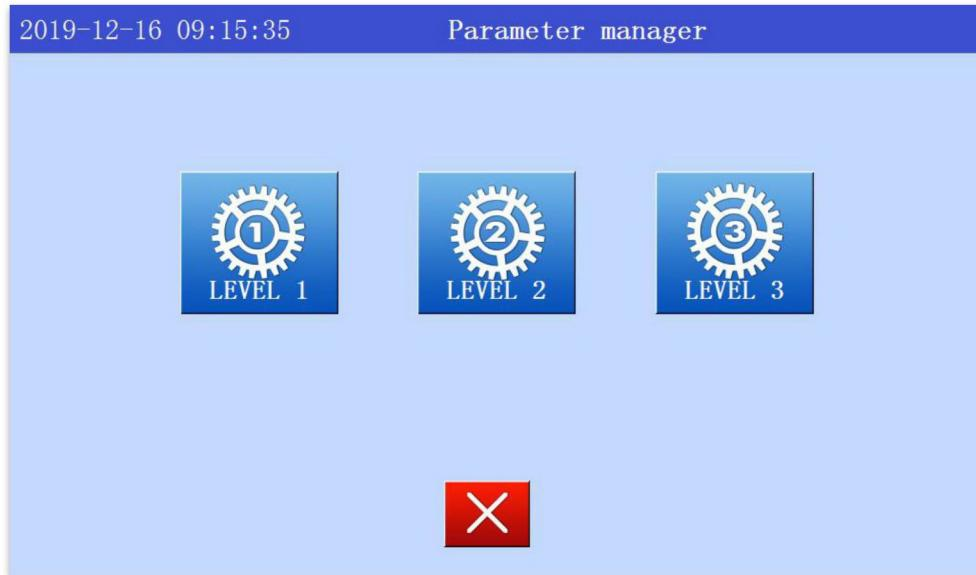
Click the key to enter the parameter list page, to see if all of the numerical display. The two and three-level parameters require a password entry. If no display, first initialize, second touch screen upgrade, and finally contact the manufacturer.
