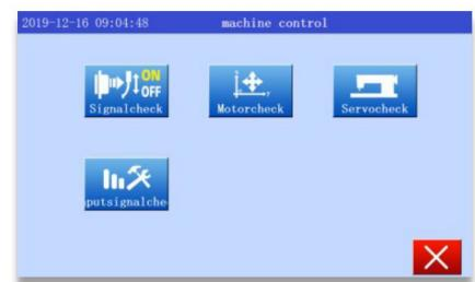
Press input Signal check key to enter the Input Signal check interface.(P20, reference Input Signal detection interface).
