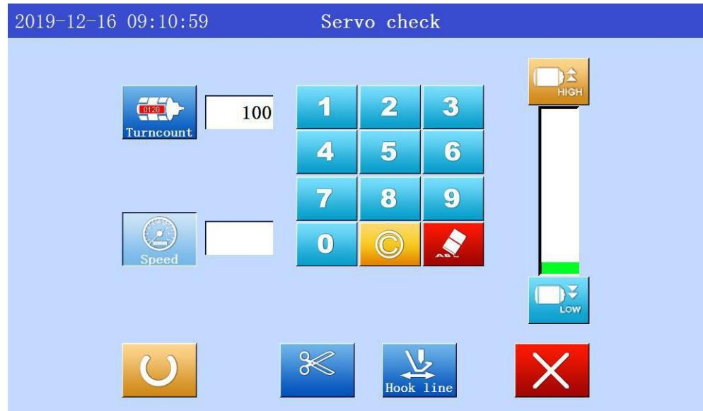
Number key input run number, progress bar side input running speed, click Run key test spindle is normal operation.
