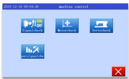
Press Electromagnetic inspection key into the Solenoid valve test Interface (P19, reference solenoid valve detection Interface).
