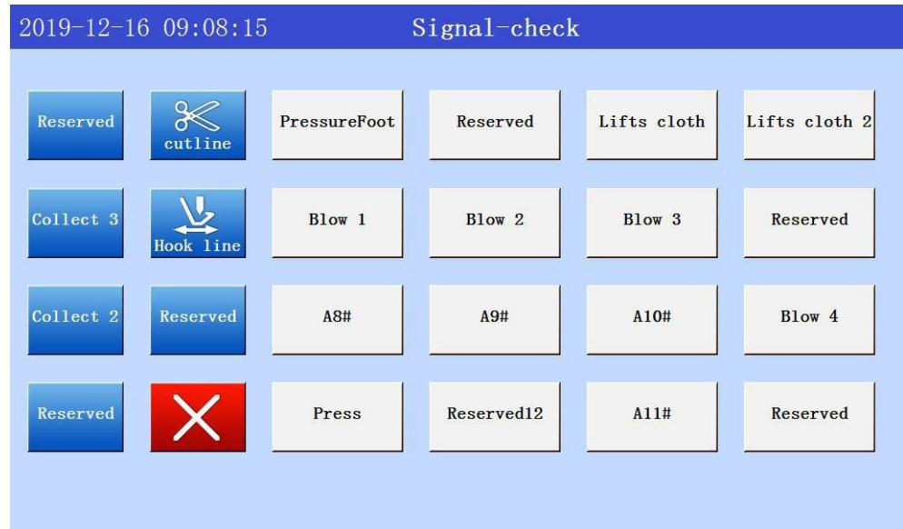
Click on the button on the interface in turn to see if the corresponding name of the part has no action, if not, to troubleshoot valve board • Solenoid valve • Trachea • Cylinder parts
