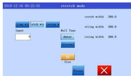
Click the button **stretch wid**, and then enter the offset of the feed width in the input Value box, with the actual value showing the width of the stretched cloth on the right.
