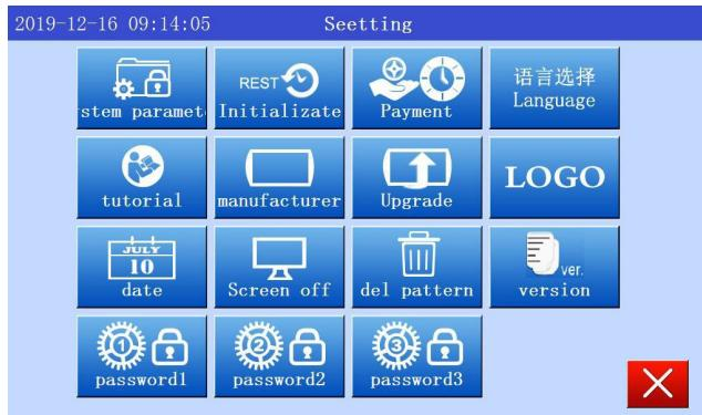
Press pattern deletion button in the Setup interface to enter the pattern delete interface. Select all patterns to delete, Press key to delete the selected patterns. Delete all patterns at once by key deleting all (P29, refer to delete the Pattern interface introduction)
