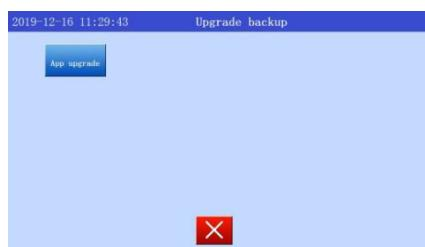
USB disk After the successful reading, click the touch **App upgrade** Screen Upgrade button to start the upgrade.
