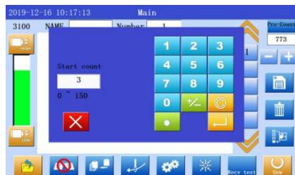
In the main control interface click the parameter box 3, enter the starting stitches number Settings page. The right keyboard to enter the actual number of pins needed, press OK
