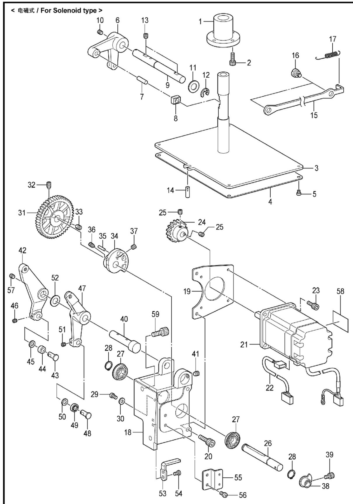
D2. 抬压装置 / Work clamp lifter mechanism
