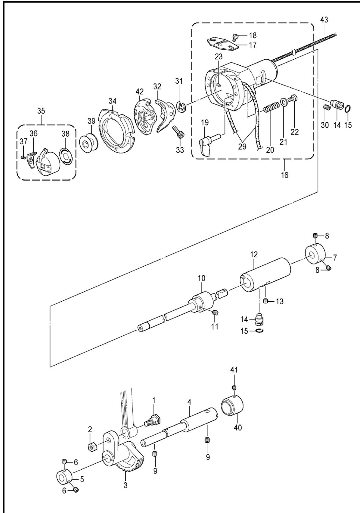
E. 下轴装置 / Lower shaft mechanism
