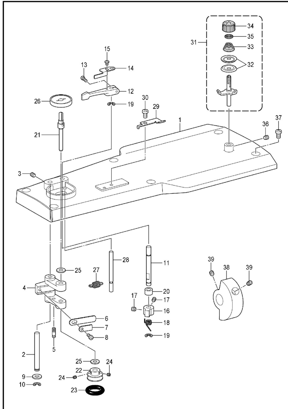
H. 卷线装置 / Bobbin winder mechanism
