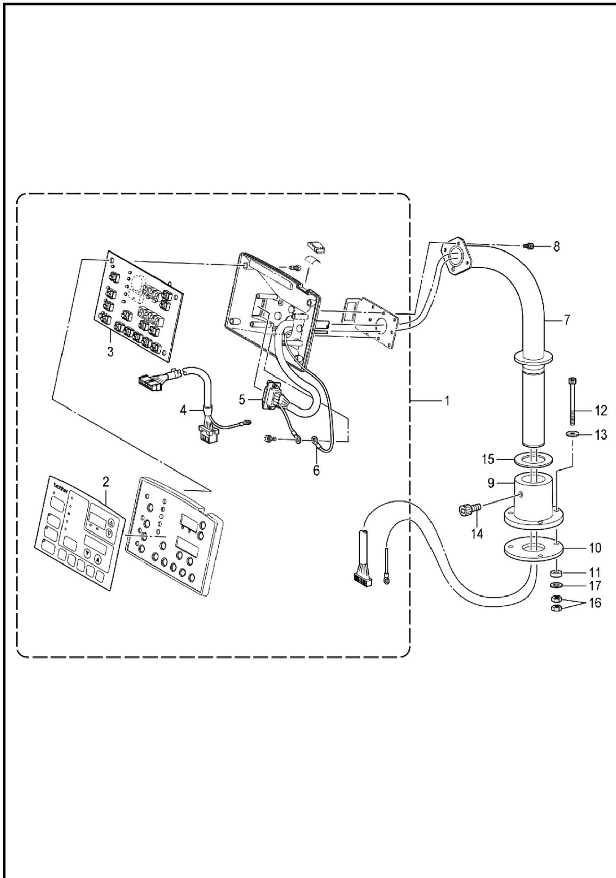
R. 操作盘装置 / Operation panel mechanism
