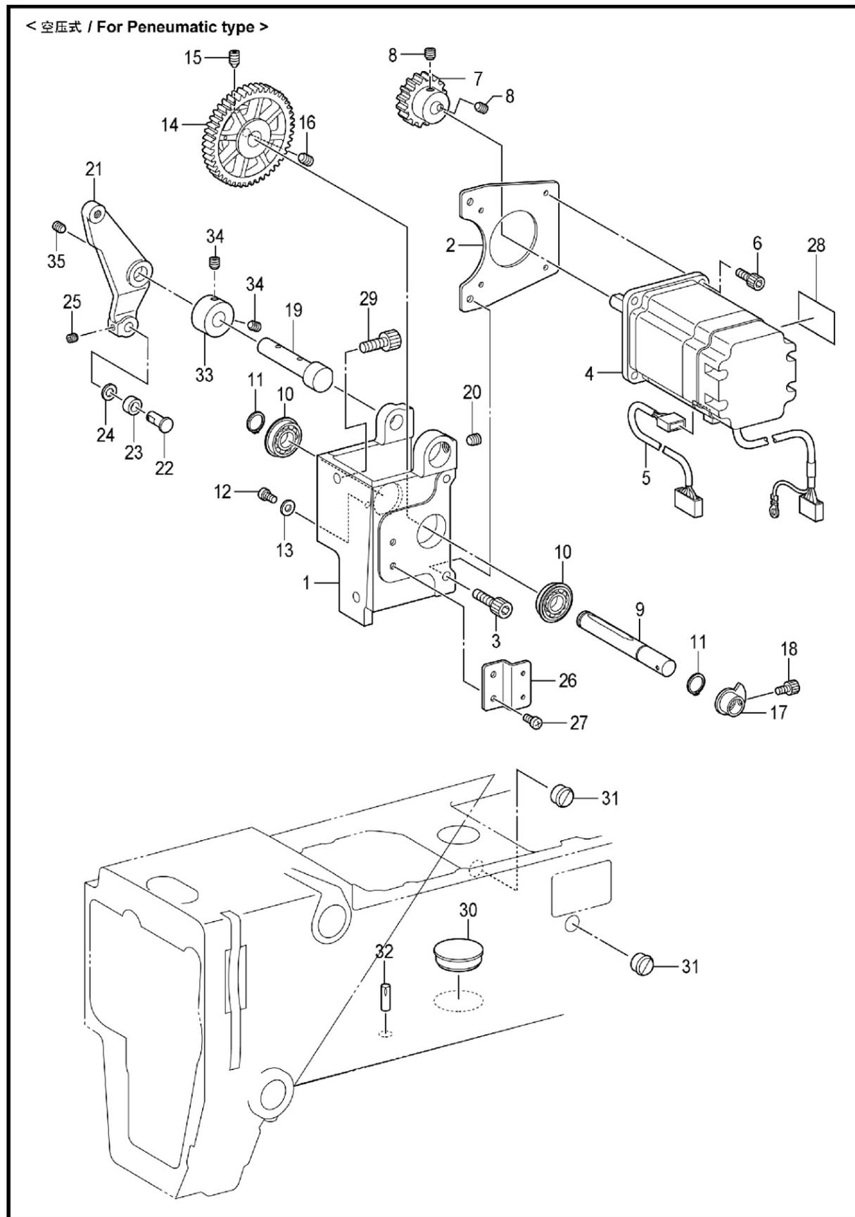
D3. 抬压装置 / Work clamp lifter mechanism
