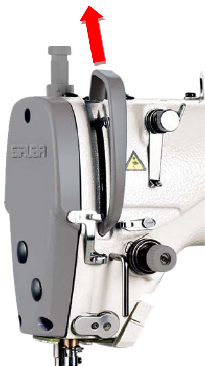
挑線桿位置示意圖 Schematic diagram of thread take-up lever
