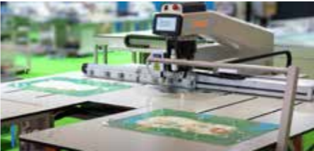
SS 双模板送料：自动换模并车缝，节省换模的人力。 Double Template Feeding Device: Automatic mold changing and sewing to save labor on mold replacement.
