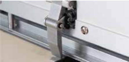
GD 固定勾装置：设备本身的压模装置外加的双层保护，确保模板固定在正确位置。 Template Fixed Clasp Device: The machine's own pressing mold device, along with double-layer protection, ensures the template is fixed in the correct position.
