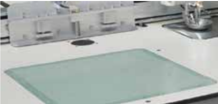
XF 吸风装置：此装置配合模板，可达到自动折边，省去熨烫的流程。 Suction Device: This device, when used with a template, can achieve automatic hemming, eliminating the need for ironing.
