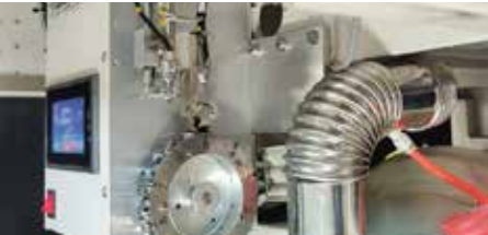
SX 自动换芯：系统内设置针数，自动停机更换梭芯，共10个梭芯(含机头上)。 Automatic Bobbin Change Device: System settings for stitch numbers, automatic shutdown for bobbin replacement, with a total of 10 bobbins (including the one on the machine head).
