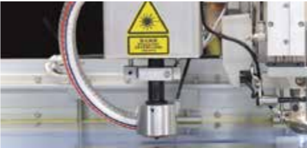
JG 雷射：用於皮/布料切割。 Laser Cutting Device: For cutting fabric and leather.
