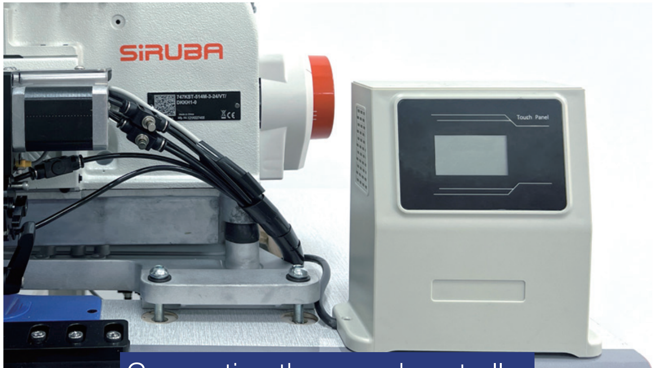
Connecting the speed controller
