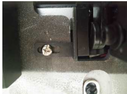
Fig.2 After the button feeder machine sensor is installed
