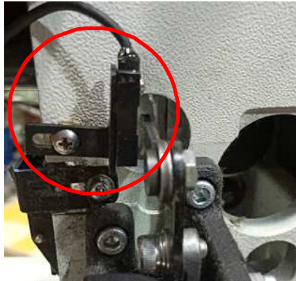
Fig.6 Installation Position of Button Sender Sensor
