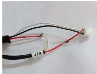
Fig. (8) Installation Position of J28 Broken Needle Protection Sensor (Protect the Button Attaching Machine)
