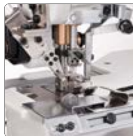
CHP (CRL 163) 氣動式下擺車縫 Pneumatic Hemming
